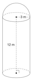
Its volume can be determined using the following formula, in which r is the radius and h is the height of the cylinder.
